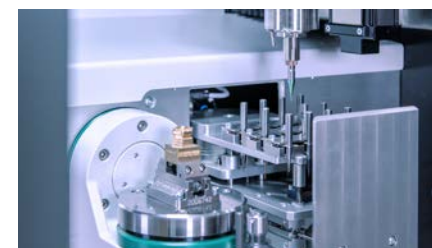
Standard tool magazine Direct clamping with twelve places
