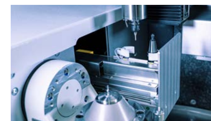
Tool changing system with a large tool storage
